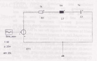
Figure 6: SIMPLORER Model of RLC Network.
