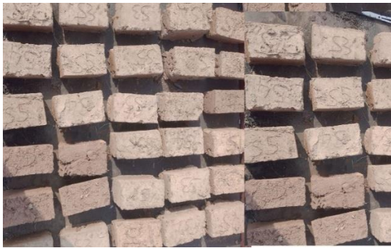
Plate 3: Bricks during sun drying and curing
