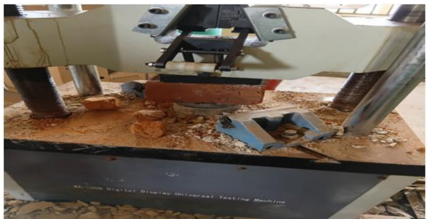
Plate 4: Bricks being crushed with compressive strength machine
