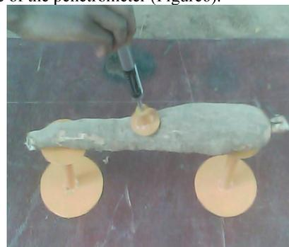
Figure 6: Determination of bioyield force
