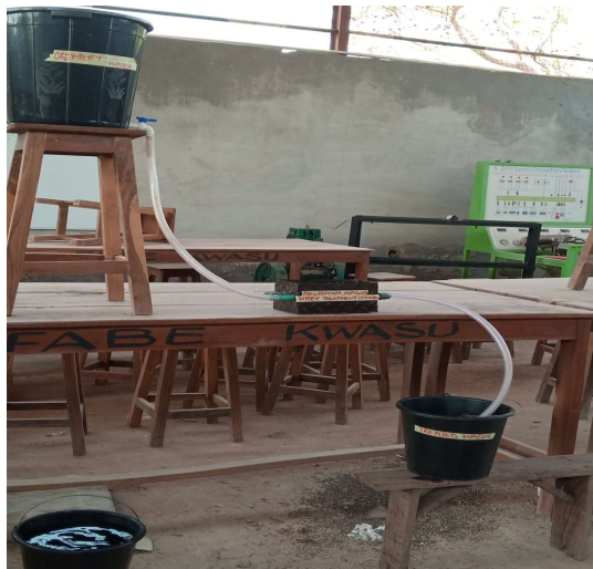
Figure 1. Magnetic water treatment set up
