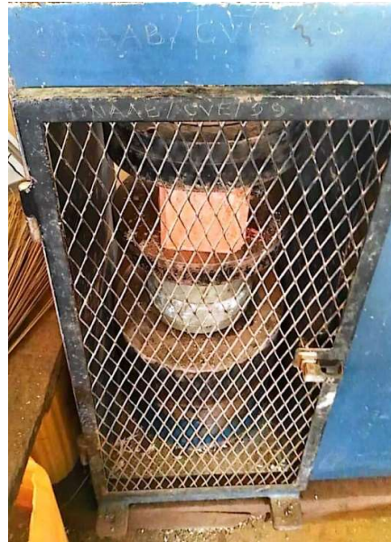
Fig 2: Testing for the comprehensive strength of the CSEBs
