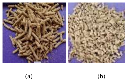
Fig. 3: pictorial view of (a) rice bran and (b) corncob pellets
