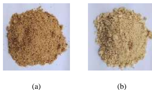
Fig. 2: Ground (a) rice bran and (b) corncob
