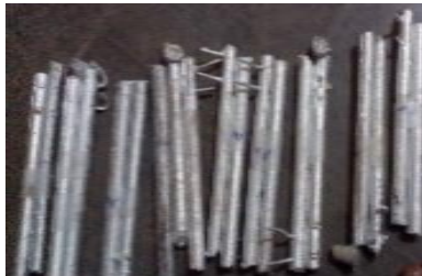
Fig.1: Samples of composites reinforced with CSA/CPA/RHA using a two-step stair casting method.
