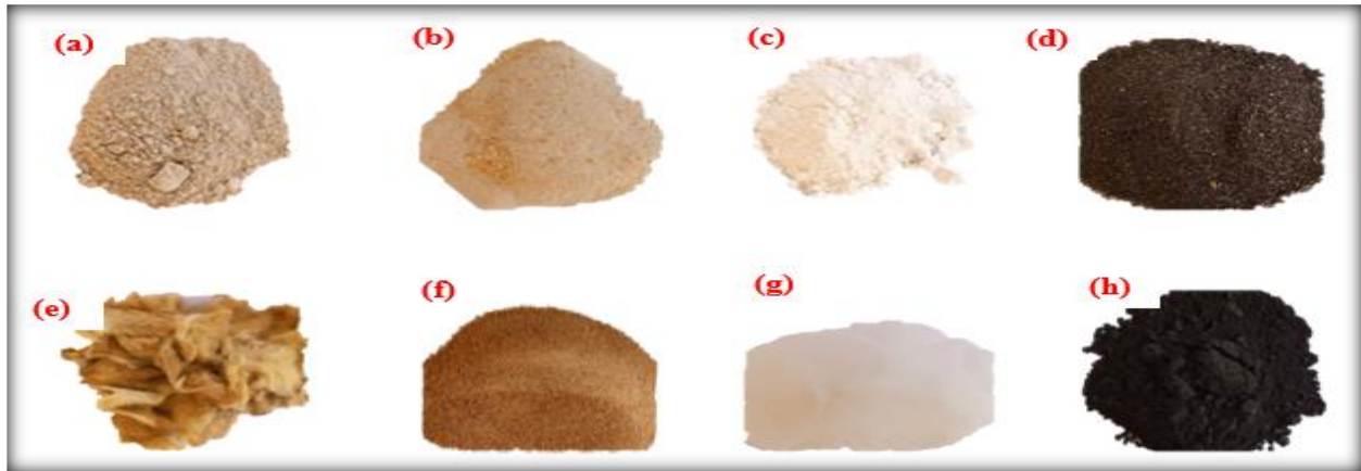
Figure 1: Filler [(a) Kaolin (c) Barium sulphate]; Binder [(b) Epoxy Resin]; Reinforcing Materials [(d) Steel fibre (e) Fibre Glass]; Abrasive Materials [(f) Silica (g) Alumina]; Lubricant [(h) Graphite].
