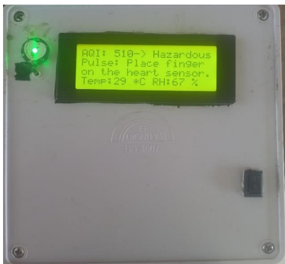
Figure 7. Prototype device of AQH-BM before the finger is placed
