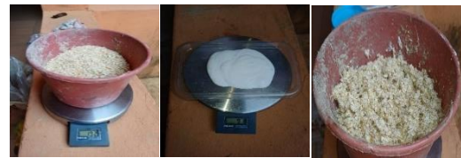
(a) Weighing of the Zmay-cob (b) Weighing of the Urea-Formaldehyde (c) material mixture
