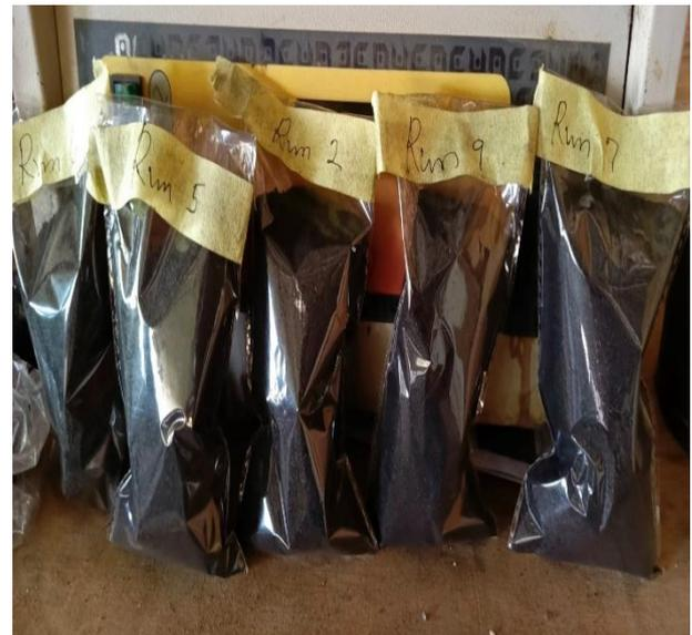
Figure 3: Bio-char obtained during the pyrolysis experiment
