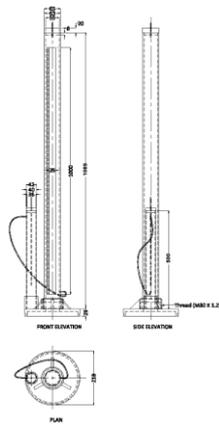
Figure 2. Details of the complete tension infiltrometer (membrane and its fastener not shown but linen scale attached to left side of the 25 mm slit is shown in the front elevation).
