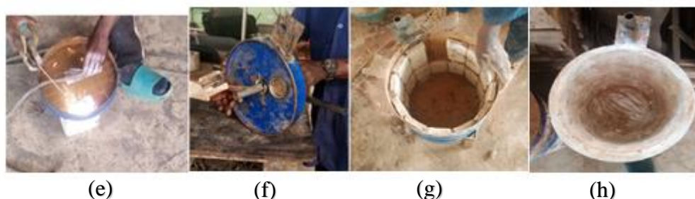
Plate 1(e-h): (e) Wire mesh welded to the lid (f) Reactor lid with pipe as vent (g) Lining the reactor with refractory clay (h) Reactor lined with refractory clay
