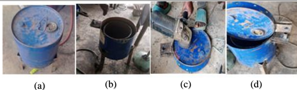
Plate 1(a-d): (a) Reactor mounted on three angled iron bar (b) Reaction chamber and the top flange (c) Reactor lid with rectangular flange (d) Reactor and lid with flange on both
