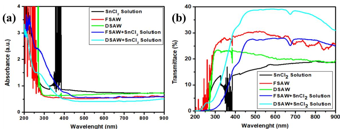
Figures 6: Absorbance-wavelength and Transmittance-wavelength plots of synthesized  $\text{SnO}_2$  nanoparticles extracted  $\text{SnCl}_2$ , FSAW, DSAW, FSAW+ $\text{SnCl}_2$  and DSAW+ $\text{SnCl}_2$
