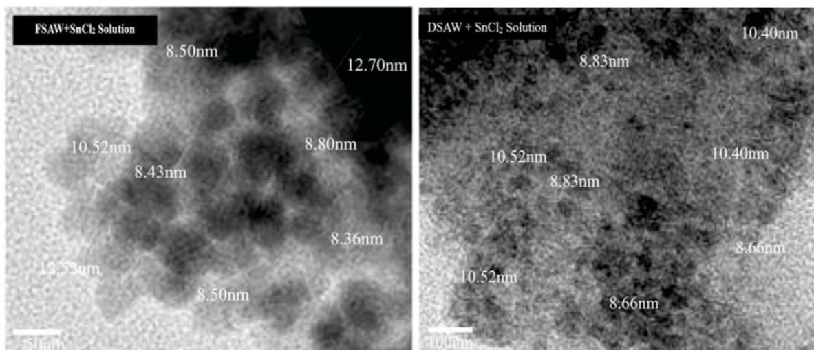
Figure 4: TEM images of synthesized SnO<sub>2</sub> nanoparticles extracted FSAW+SnCl<sub>2</sub> and DSAW+SnCl<sub>2</sub>
