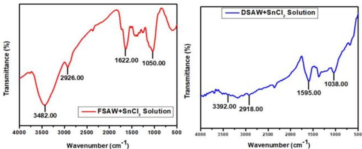
Figure 2: FTIR spectra of synthesized SnO<sub>2</sub> nanoparticles extracted FSAW+SnCl<sub>2</sub> and DSAW+SnCl<sub>2</sub>
