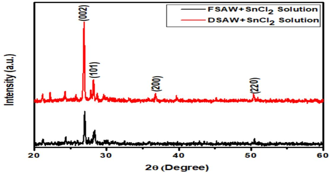
Figure 1: XRD patterns of synthesized SnO<sub>2</sub> nanoparticles extracted FSAW+SnCl<sub>2</sub> and DSAW+SnCl<sub>2</sub>
