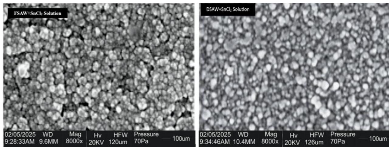
Figure 3: SEM images of synthesized SnO<sub>2</sub> nanoparticles extracted FSAW+SnCl<sub>2</sub>, and DSAW+SnCl<sub>2</sub>
