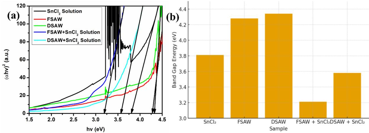
Figures 7: Absorption coefficient-energy gap plots and variation of optical band gap of synthesized SnO<sub>2</sub> nanoparticles extracted: SnCl<sub>2</sub>, FSAW, DSAW, FSAW+SnCl<sub>2</sub> and DSAW+SnCl<sub>2</sub>.
