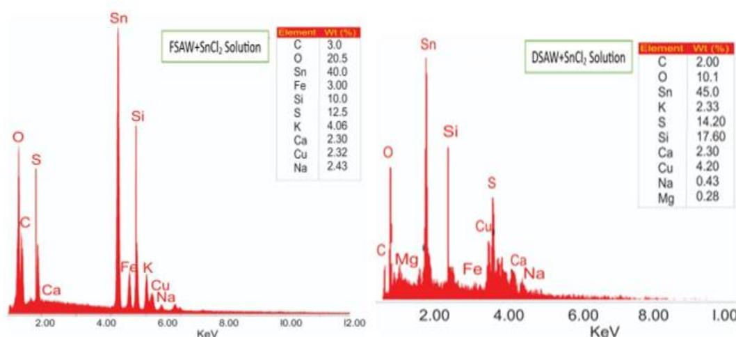
Figure 5: EDX Spectra of synthesized SnO<sub>2</sub> nanoparticles extracted FSAW+SnCl<sub>2</sub> and DSAW+SnCl<sub>2</sub>
